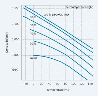
Figure 8: Density of aqueous LIPOXOL solution as function of temperature
