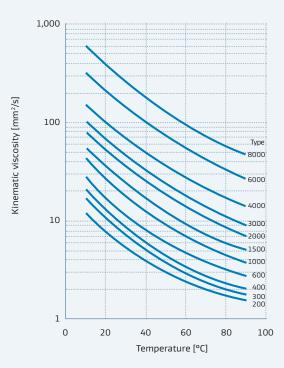
**Figure 3:** Kinematic viscosity of LIPOXOL grades (50% LIPOXOL in aqueous solution)
