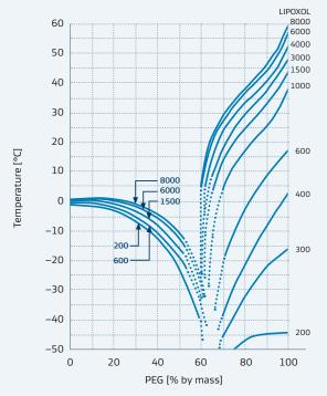
Figure 6: Solidification temperature of aqueous LIPOXOL solution
