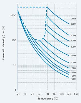
Figure 2: Kinematic viscosity of LIPOXOL grades
