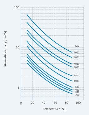
**Figure 4:** Kinematic viscosity of LIPOXOL grades (30% LIPOXOL in aqueous solution)
