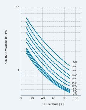
**Figure 5:** Kinematic viscosity of LIPOXOL grades (10% LIPOXOL in aqueous solution)
